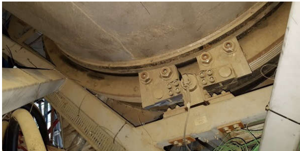
FIGURE 9. Dust on bearing
