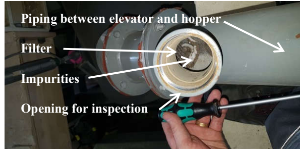
FIGURE 10. Impurities in particles clogging a filter
